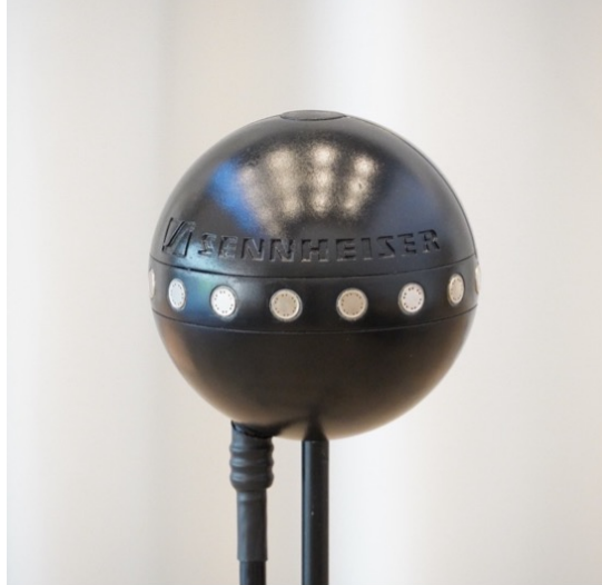
Figure 9: 16-channel equatorial microphone array with a diameter of 16 cm that produces 7th-order ambisonics. The hardware design is described in (Fiedler, 2018). Find a demo of it here 4 . (Photo: Jens Ahrens)
