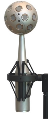
Figure 8: Photograph of the commercial spherical microphone em32 Eigenmike™ with 32 channels and a diameter of 8.4 cm. It can deliver a 4th-order ambisonic signal. (Photograph: Jens Ahrens)
