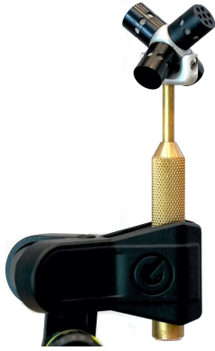
Figure 7: Photograph of a commercial tetrahedral microphone. It is composed of four nearly coincident outward-facing cardioid-like capsules. It can deliver a 1st-order ambisonic signal. The head with the microphone capsules has a diameter of approx. 4 cm. (Photograph: Jens Ahrens)
